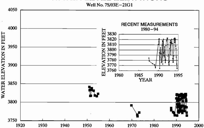
Ground El. 3863 Ft Depth 260 Ft Perf 20 – 260 Ft Drilled in Old Alluvium Anza Mutual Water Co. Well No. 1 (1987–1994) DWR Bulletin 91–22 (1950–73) dated 8/74
