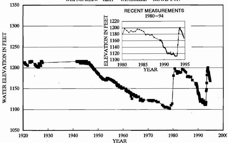
Ground El. 1216 Ft. Depth 515 Ft. Drilled in Alluvium Ref: DWR Bul 91-20 (1920-67) RCWD Master Plan (1970-83); LH Rpt (1983-87); RCWD Reports (1989-94)
