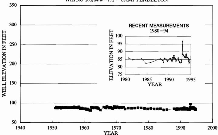
Ground El. 93 Ft Depth 138.8 Ft Perf Unknown Drilled in Alluvium Camp Pendleton Records (1950-1972)(1988-1994) LH Study (1973-85) dates estimated
