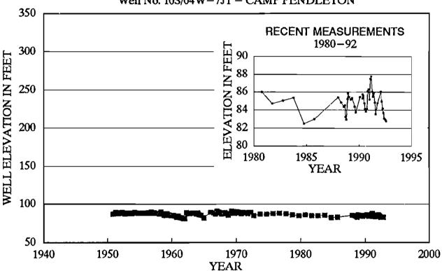
Ground El. 93 Ft Depth 138.8 Ft Perf Unknown Drilled in Alluvium Camp Pendleton Records (1950–1972)(1988–1992) LH Study (1973–85) dates estimated
