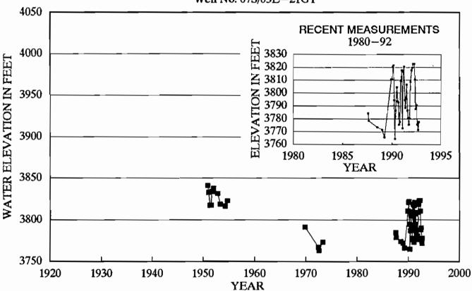
Ground El. 3863 Ft Depth 260 Ft Perf 20--260 Ft Drilled in Old Alluvium Anza Mutual Water Co. Well No. 1 (1987-1992) DWR Bulletin 91-22 (1950-1973) dated 8/74
