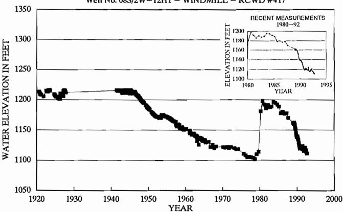
Ground El. 1216 Ft. Depth 515 Ft. Drilled in Alluvium Ref: DWR Bul. 91-20 (1920-67) RCWD Master Plan (1970-83); LH Rpt (1983-87); RCWD Reports (1989-92)
